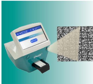
Configure the reader scanning a Datamatrix with all the features of your method.
